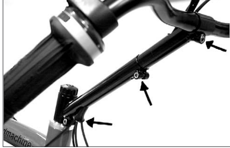
On the stem you will find 3 clamping screws for adjustment.
