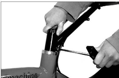
After undoing the stem clamping, you can adjust the damping.
