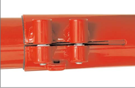
The rear end of the front boom may never be visible in the clamping slot.
