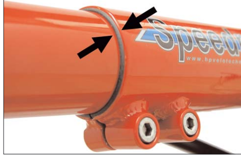
The plastic spacer between front boom and main frame must be visible at all time.
