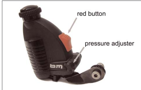
You switch on the tire dynamo by pressing the red button. To switch off the dynamo move it away from the wheel.
