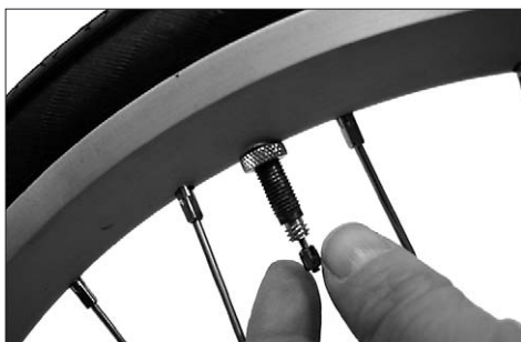
Before pumping up the tire, you have to unscrew the little knurled nut on the valve.
