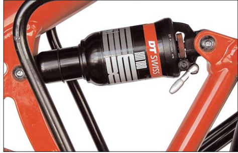
Air Shock DT-Swiss XM180. Damping is adjusted with the red knob at the rear end. The shock must be installed with the lock-out lever facing down to avoid a collision of lever and frame when the suspension is moving.
