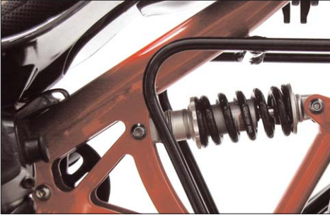
Suspension element DV-22 with fixed damping rate.
