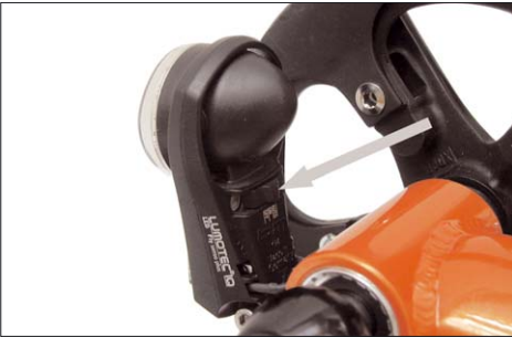
The hub generator lighting system can be set to on, off or automatic (Sensor) with the integrated switch at the front light.
